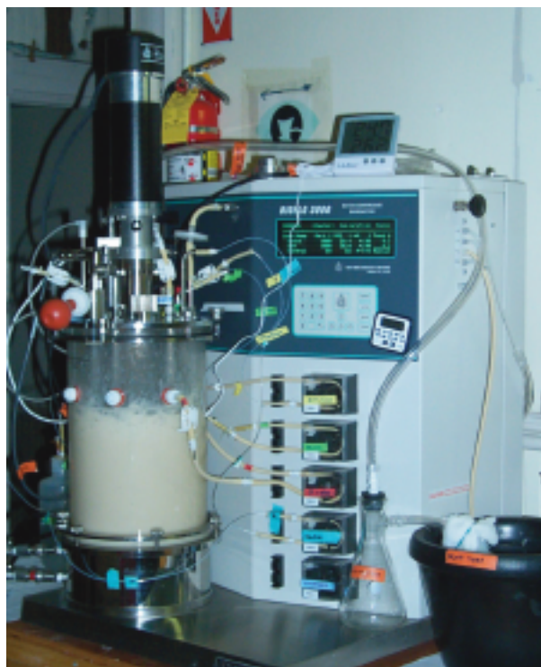
Figure 2 Nitrate reductase producing Pichia pastoris cell line grown in a BioFlo 3000 ® 14-L fermenter (New Brunswick Scientific Co., Edison, NJ).
